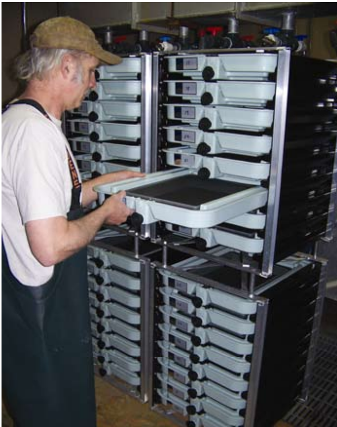
Assistant Hatchery Manager, Mark Thomas inspects the Heath trays at Trail Lakes Hatchery.
