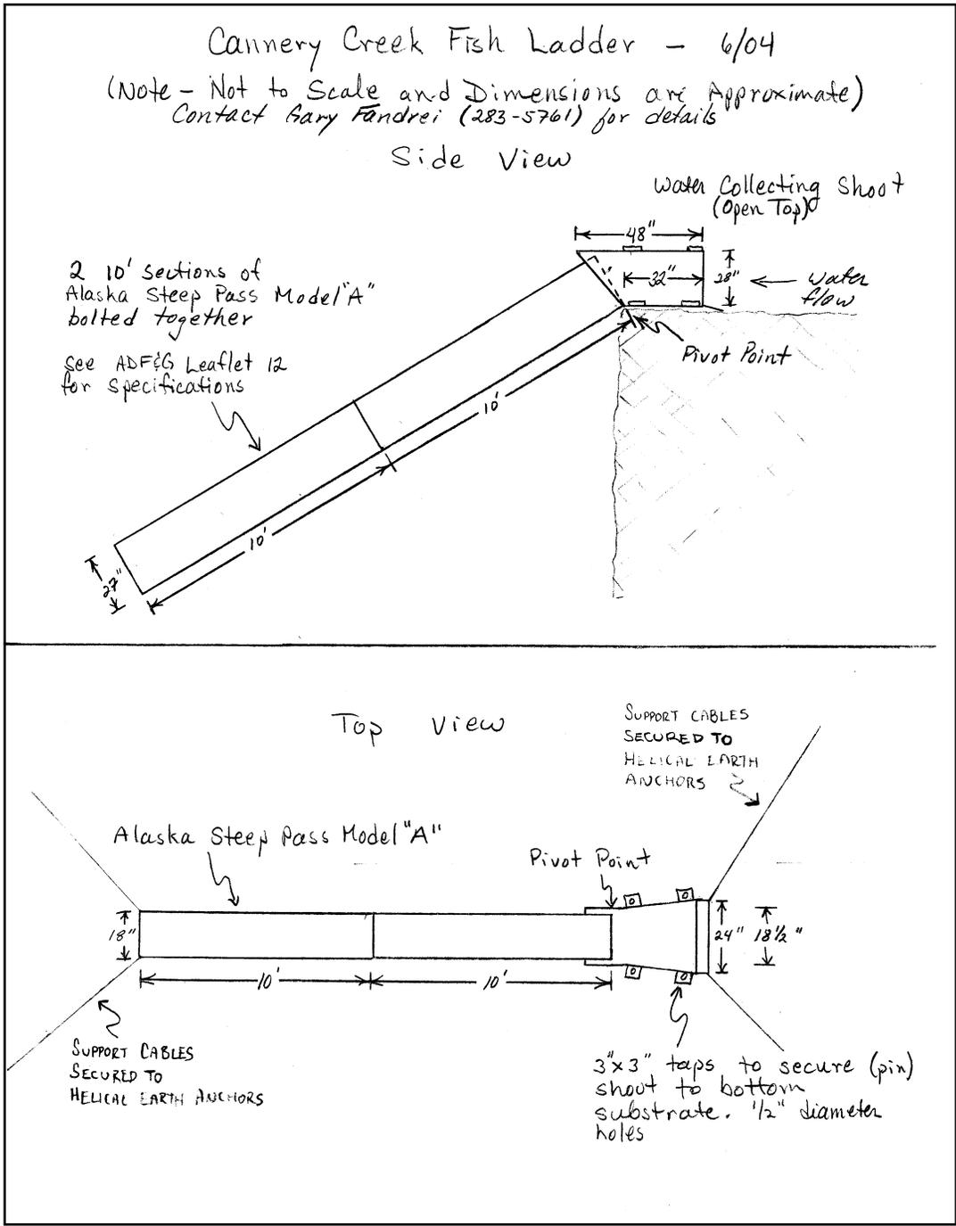
Figure 2. Sketch of Alaska Steeppass used at Cannery Creek. Note that the plans were changed from two 10ft sections to three 8ft sections.
