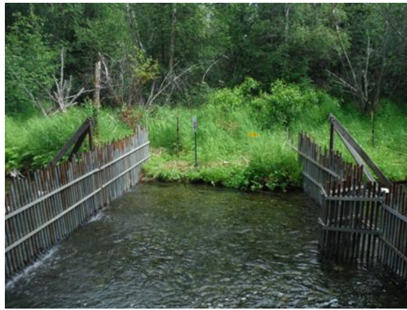
Figure 5: Trap Weir, two rows of pickets and no live box. By removing a few downstream pickets salmon can be let into the weir and then be scooped out to be sampled, easier than getting them into the live box.
